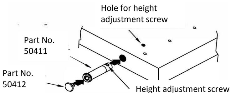
Place the height adjuster (Part No. 50411) on the underside of the unit. The height adjustment screws must match up with the holes on the side of the units. Insert glider plug (Part No. 50412).
