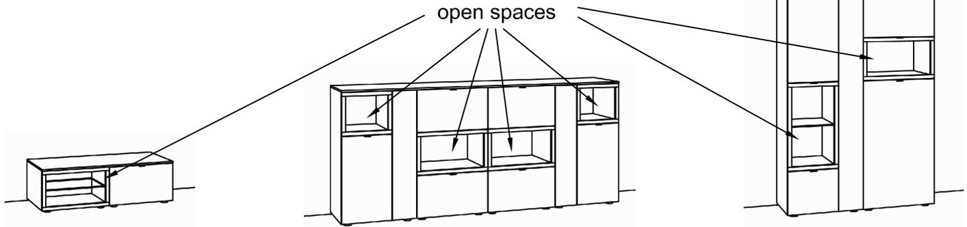
1. Our open spaces are complete inserts. They are bolted with the carcass ground / carcass side. If you want to take out the inserts, you have to unfix the screw. Now you can take out the insert. Regarding the models with lighting please pay heed to the connector cable on the back of the furniture.
